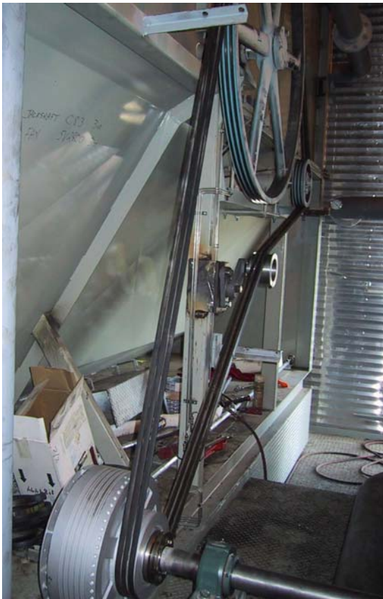
< 1000HP Gas Engine Driven remote Gas Compressor application with jackshaft mounted 50 HP "Smart Pulley" (Self-Powered) for automatic variable speed control of the unit's main cooling fan, Alberta, Canada
